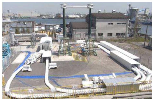
Fig. 13: View of DC320kV prequalification test loop
