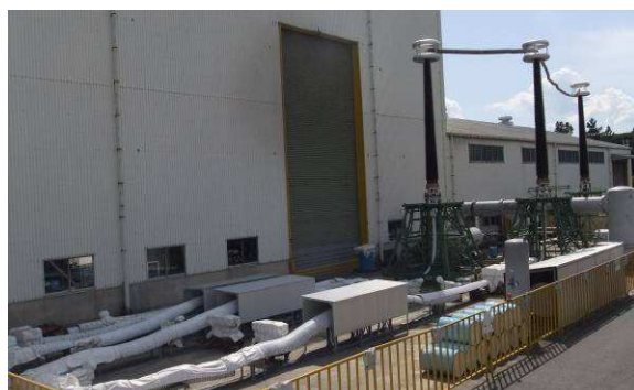
Fig. 16: View of DC320kV type test loop
